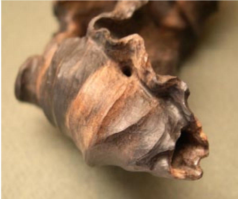
This shows the tip rolled in on itself with thinning progressing.
