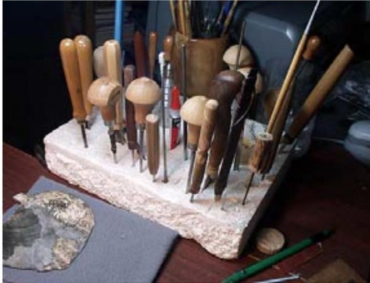
(by sergey\_osipov) I use the piece of foam plastic for placing my chisels. This very comfortable to stick chisels. There is no need to have the special place for each chisel, possible just stick the chisel in any place. Besides this saves tools from desharpening.
