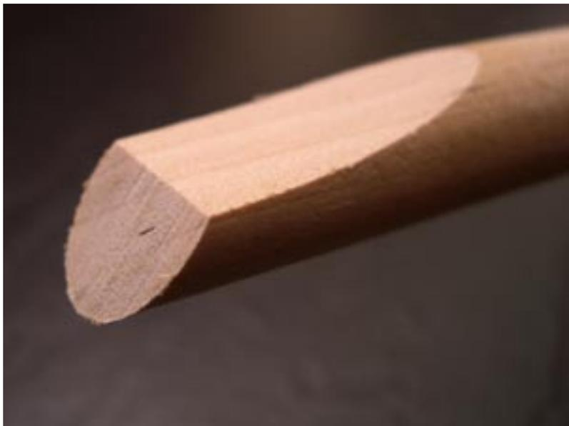
The next step is to grind the top down to reduce the size of the face and make it a more useful shape.
