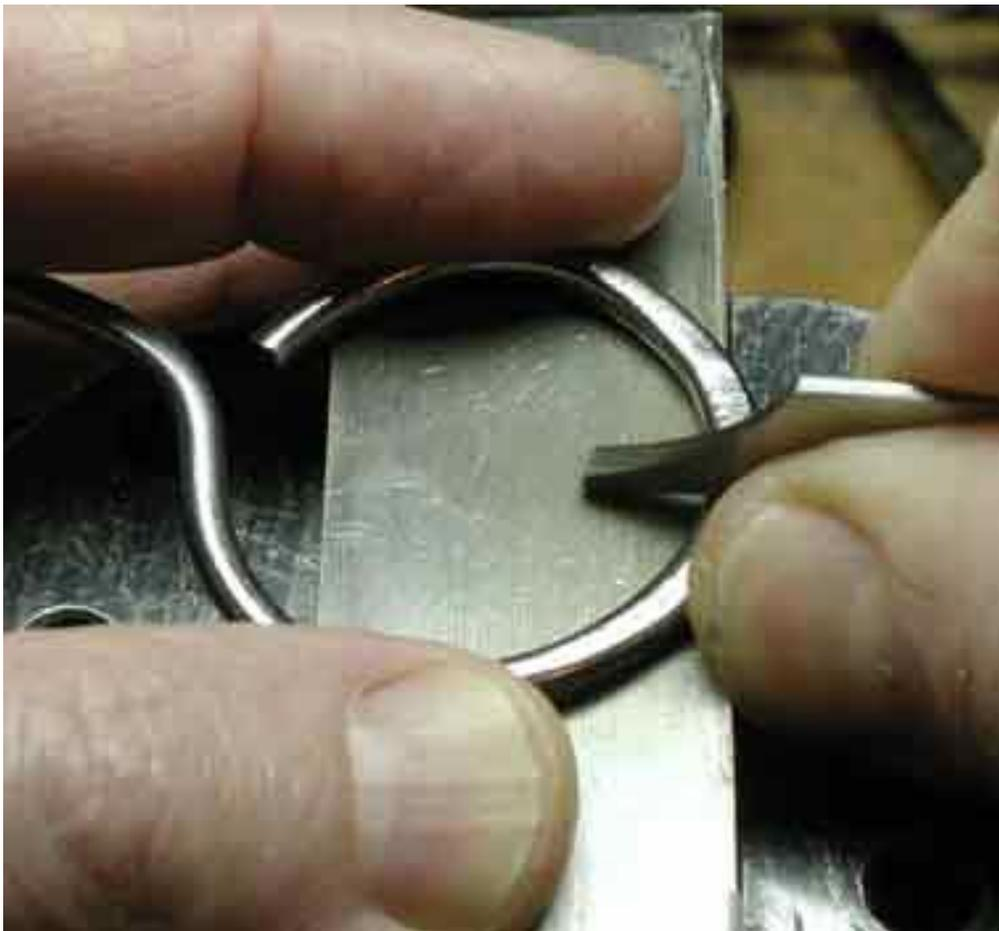
Here is a picture of a tool I use a lot. It's a type of fulcrum for my gravers. It works best with flat or round gravers, but not well with onglettes and knives. I hold the tool with my left hand, and rest the graver on it right behind the tip. The graver rides on the ring, and enables me to get great control, and lots of power. I can scrape small amounts of metal, or large amounts depending on how
