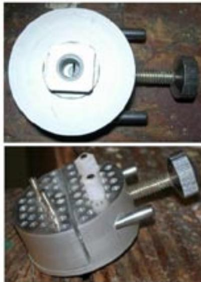
(by E George) I have a Peg Vice. It is useful for some work. The wooden handle can be removed and there is a small square plate on the bottom of the clamp which can be held in a small vice ( I hope the attached picture is correct size and shows this plate). The result is a poor man's engravers block.
