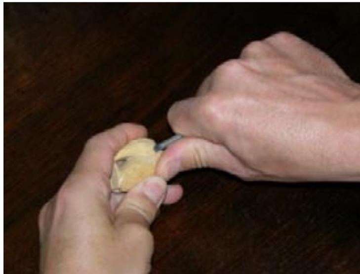
(by Ko Baas) I never use any holding device. Just hold the piece in my left hand and the tool in my right. Mostly as you would hold a hammer, sometimes with delicate work as you would hold a pencil. I move the workpiece just as much as the tool. With combined movements.
